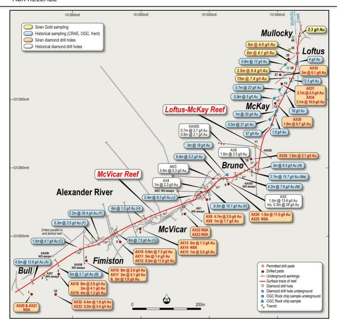
Figure 2. Plan of the trench and drillhole intersections.
