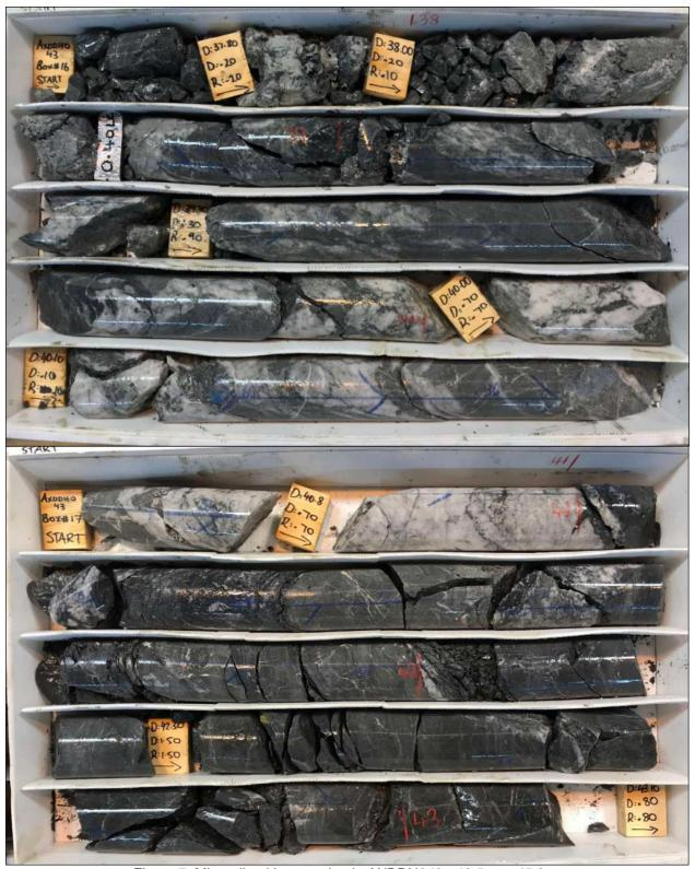
Figure 7. Mineralised intersection in AXDDH043 - 42.5m to 45.0m.
