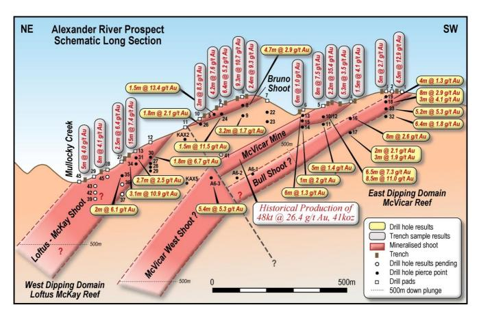
Figure 1. Schematic long section through Alexander reef system.
