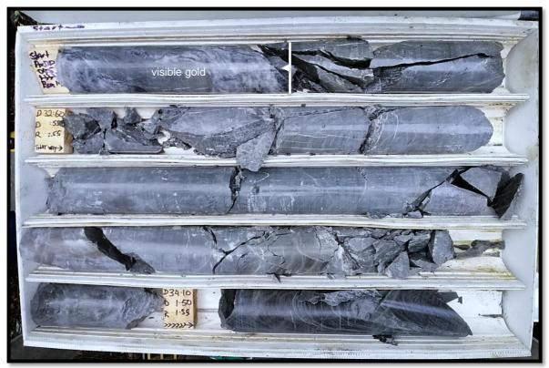
Figure 3. AXDDH045 core showing the mineralised reef between 30.9m and 32.7m.
