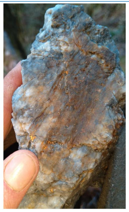
Figure 5. Quartz Reef with significant visible gold in the Victory United reef.
