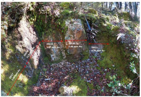
Figure 7. A2 quartz reef outcrop and channel samples results.
