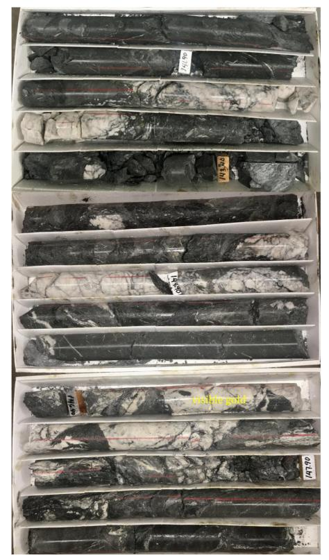
Figure 14. Quartz reef intersected in Big River BRDDH027 between 142 and 148m with visible gold at 146.7m.
