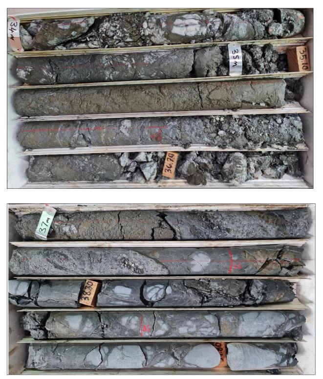
Figure 12. Core from BRDDH023 showing quartz breccia and massive sulphide for 5m from 33-38m.
