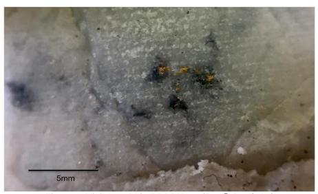
Figure 3. Visible gold in BRDDH027 (5m @ 5.1g/t Au)
