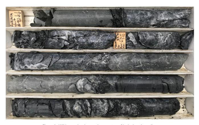
Figure 3. AX74 core showing smokey quartz reef in the hangingwall.
