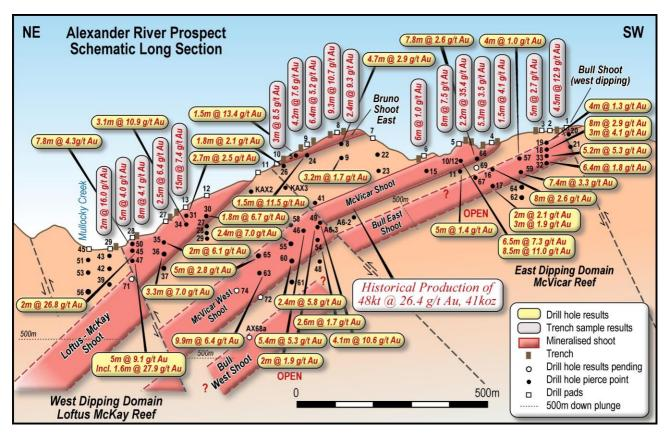
Figure 1. Schematic long section through Alexander River reef system.
