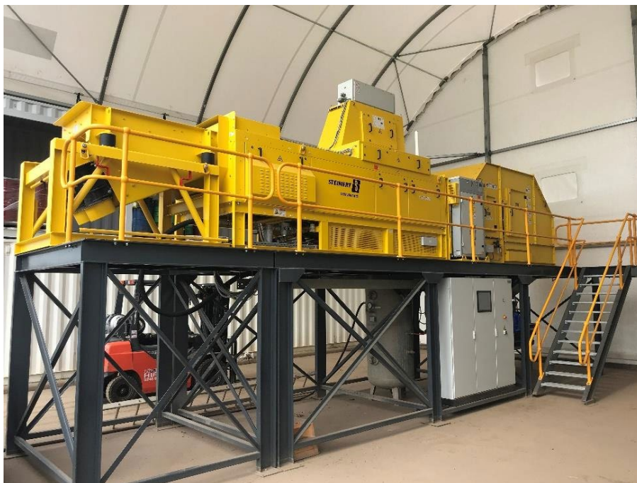
Figure 7: KSS FLI XT Sensor Sorter at STAU's test facilities in Bibra Lake
