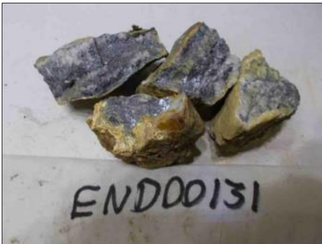
Figure 7. Stibnite bearing ore from the mullock heap below adit No1 at 440mRL (Green 2015).
