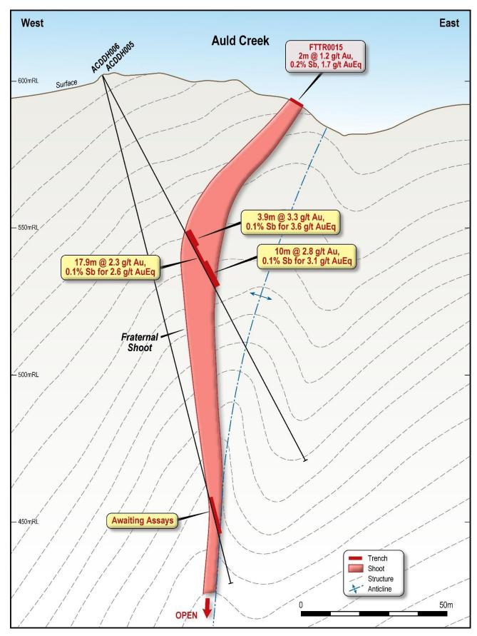
Figure 4. Cross section through ACDDH005 and ACDDH006.
