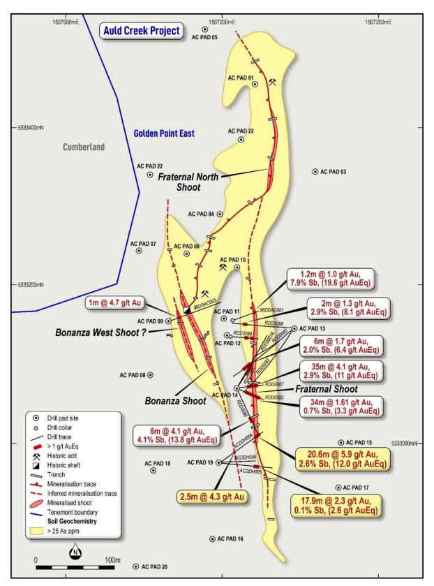
Figure 2. Auld Creek drillhole plan
