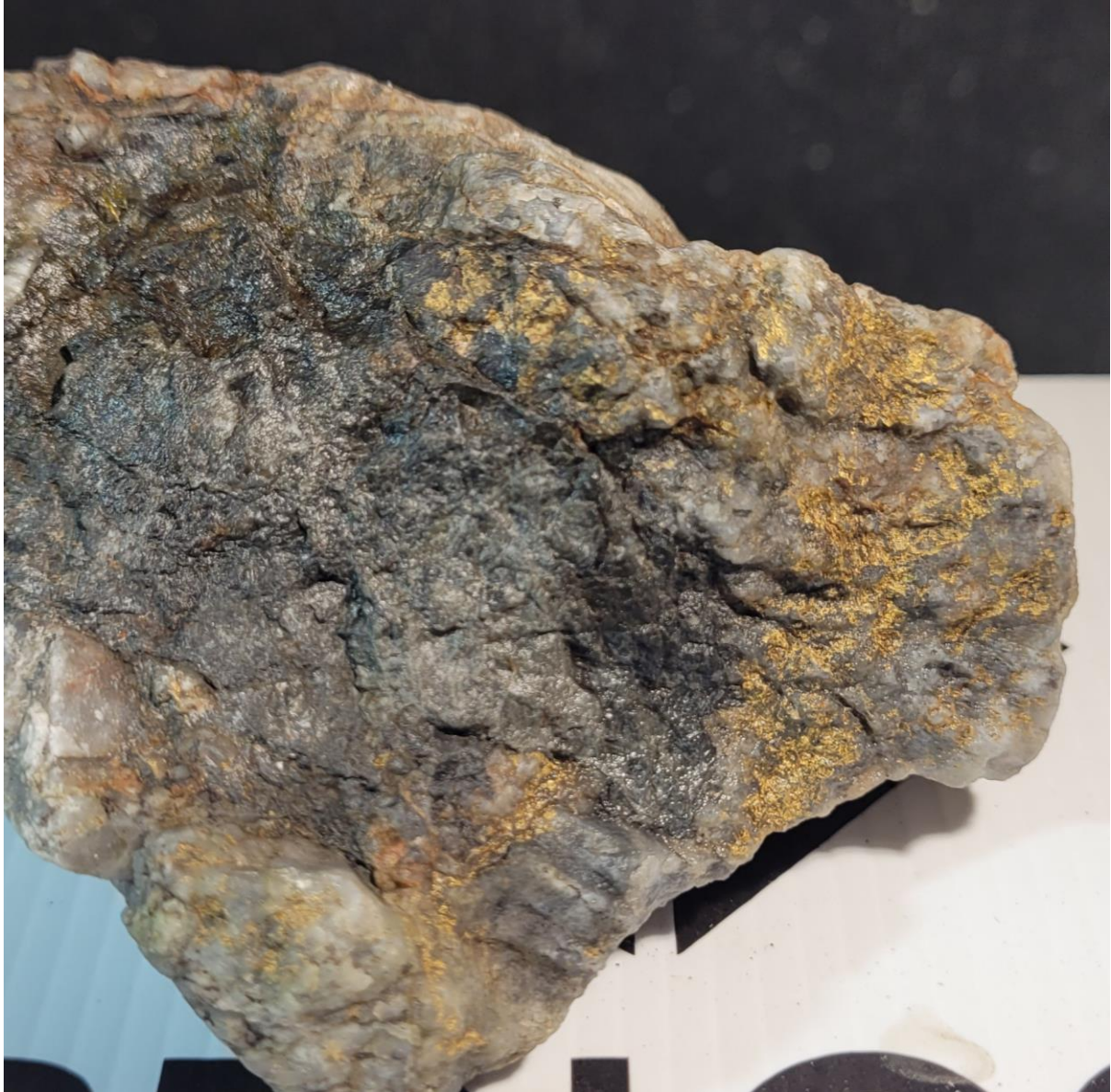
Figure 7. Significant visible gold in a float sample from the historic McVicar mine.
