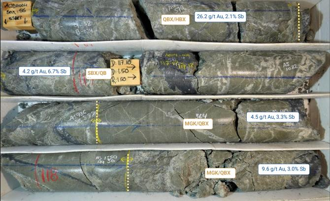
Figure 5a. Fraternal Shoot intersected in AXDDH004 116.2m – 118.4m. (SBX - stibnite cemented breccia, QBX – quartz breccia, HBX – host rock breccia, MGK – silicified disseminated arsenopyrite mineralised greywacke, MAR - silicified disseminated arsenopyrite mineralised argillite).
