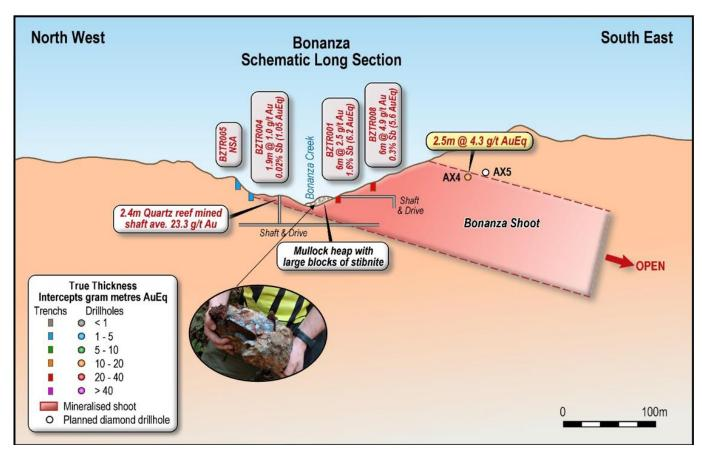
Figure 6. Bonanza N-S schematic long section.
