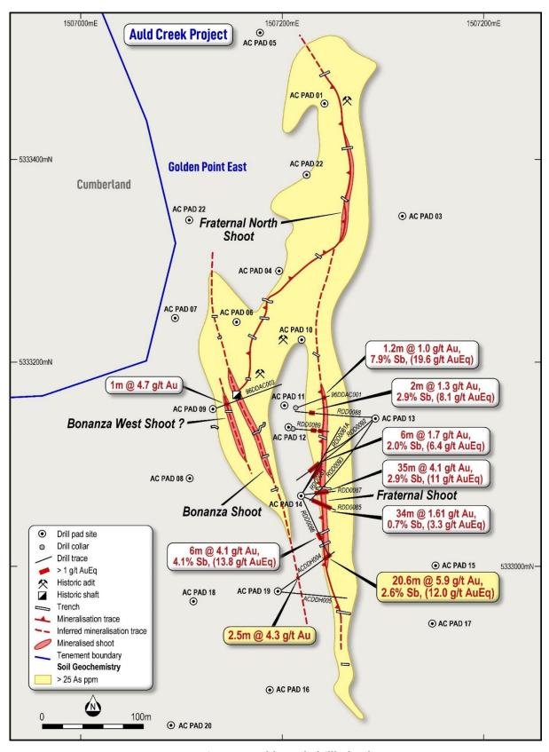
Figure 2. Auld Creek drillhole plan.
