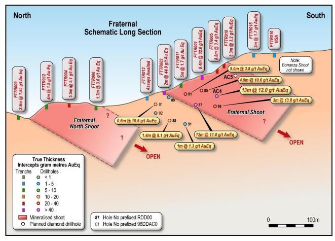
Figure 3. Fraternal N-S schematic long section.
