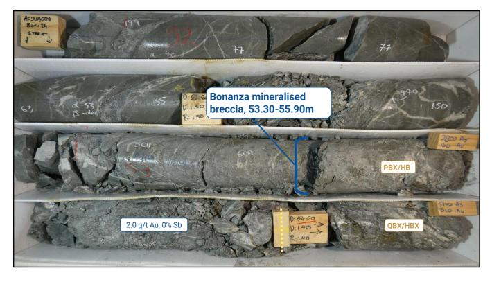
Figure 7a. Bonanza Shoot intersected in AXDDH004 53.3m – 54.2m (SBX - stibnite cemented breccia, QBX – quartz breccia, HBX – host rock breccia, MGK – silicified disseminated arsenopyrite mineralised greywacke, MAR - silicified disseminated arsenopyrite mineralised argillite.
