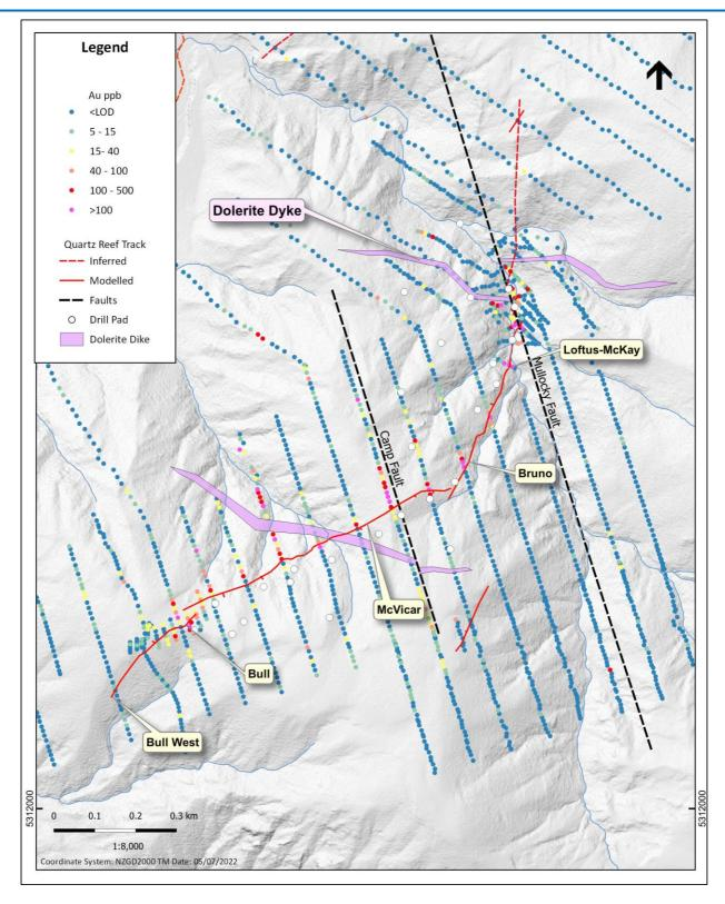
Figure 5. Dolerite dike and reef track potentally offset along the Mullocky Fault.
