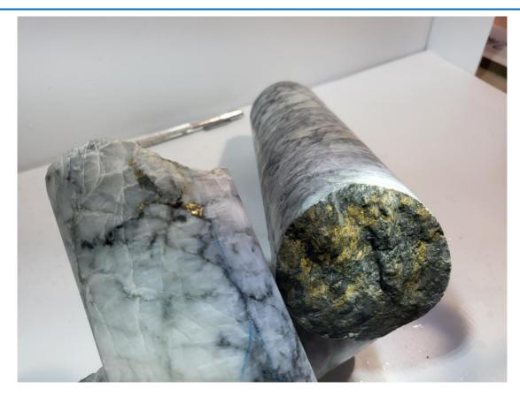
Figure 3. Significant visible gold intersected in the McVicar West Shoot in AX84.
