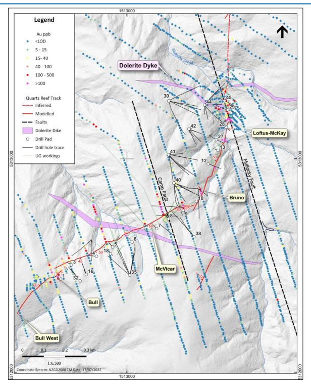
Figure 1. Dolerite dike and reef track potentially offset along the Mullocky Fault.
