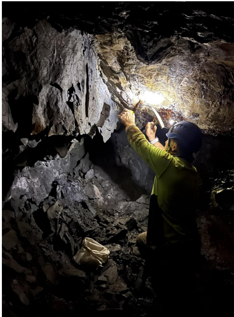
Figure 6. Sampling the quartz reef in St George Level 1 adit
