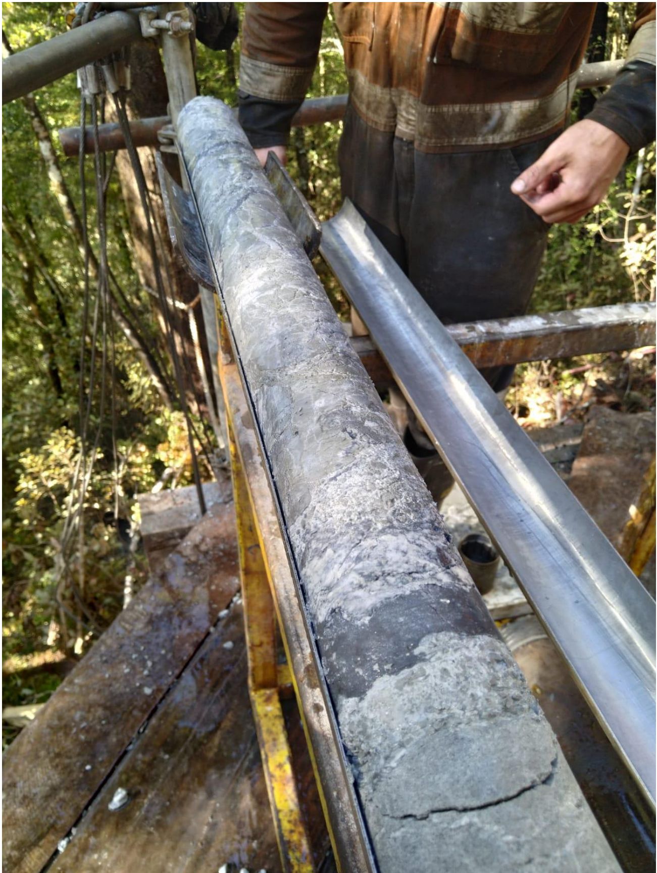
Figure 5. Stibnite cemented breccia at the top of the Fraternal Shoot.
