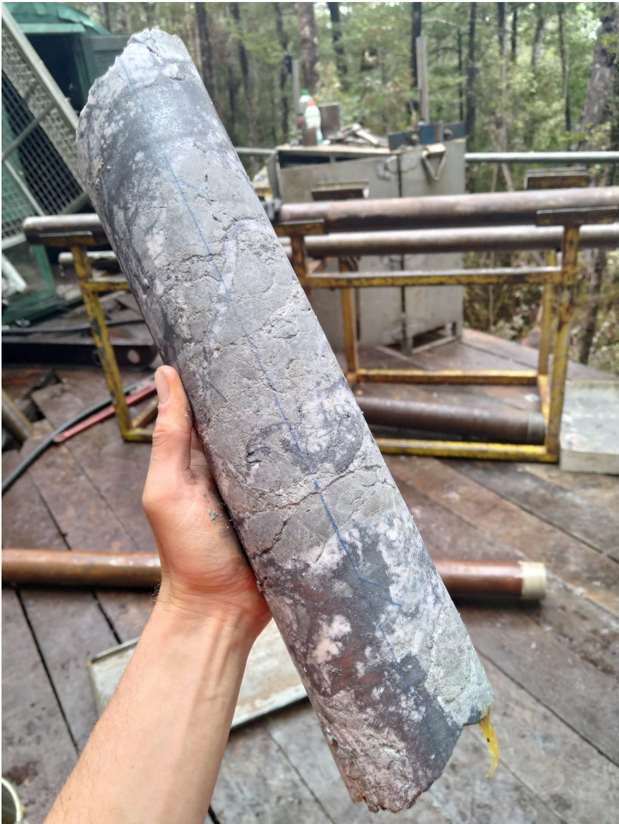
Figure 1. Stibnite (black) cemented host rock breccia from ACDDH004 at 118.6m.
