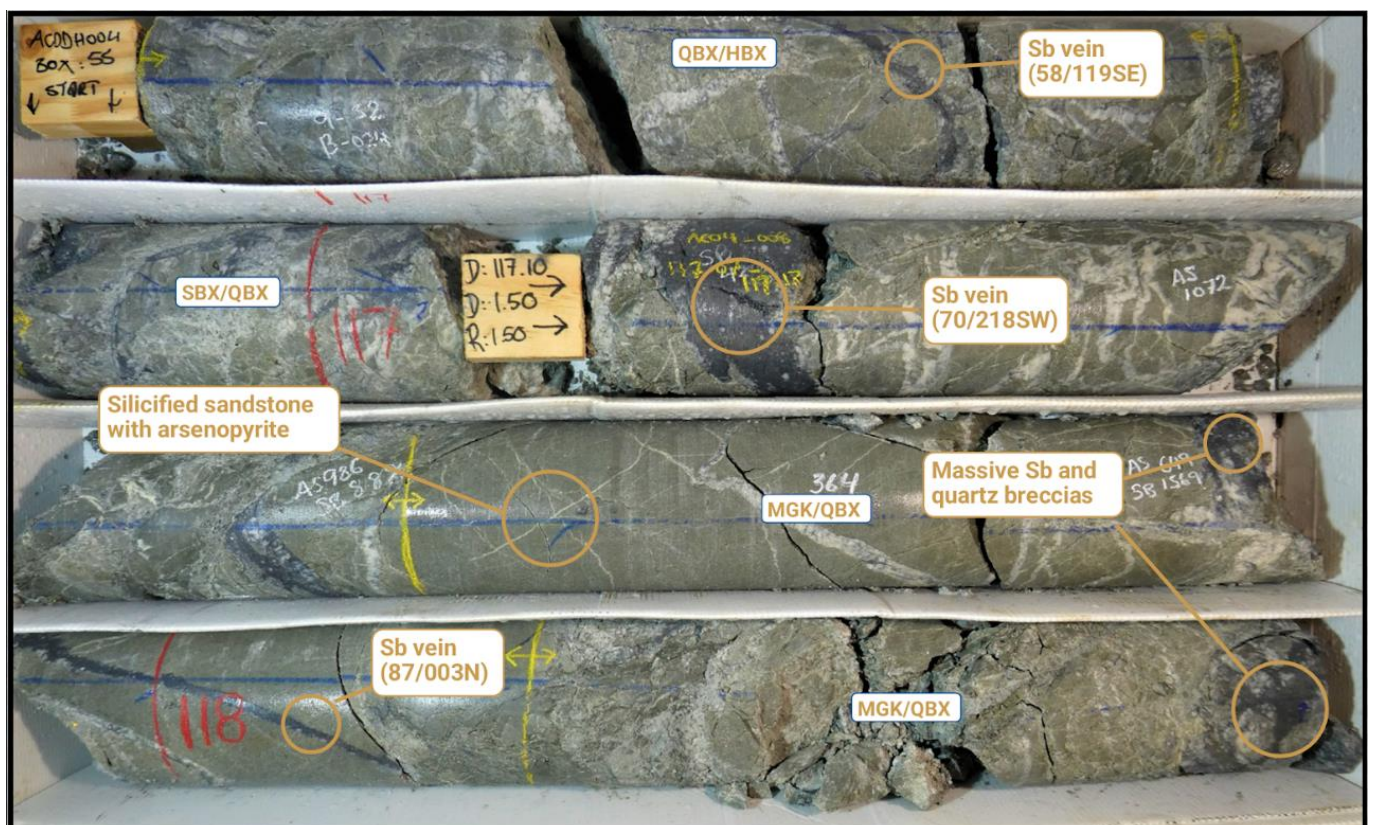
Figure 6a. Fraternal Shoot intersected in AXDDH004 116.2m – 118.5m (SBX - stibnite cemented breccia, QBX – quartz breccia, HBX – host rock breccia, MGK – silicified disseminated arsenopyrite mineralised greywacke, MAR - silicified disseminated arsenopyrite mineralised argillite).
