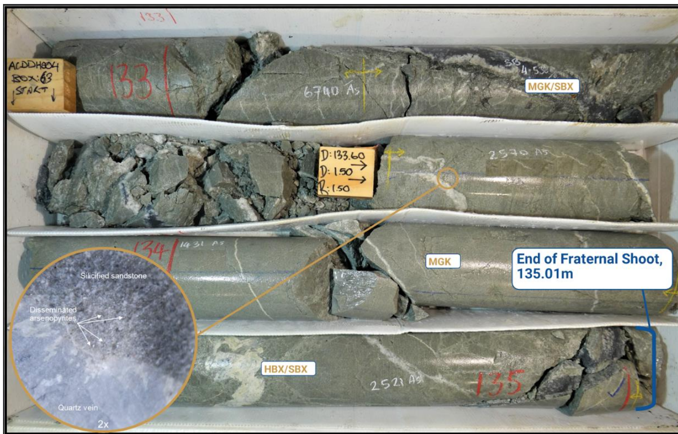
Figure 6e. Fraternal Shoot intersected in AXDDH004 130.9m – 135.0m. Inset photo = acicular arsenopyrite crystals
