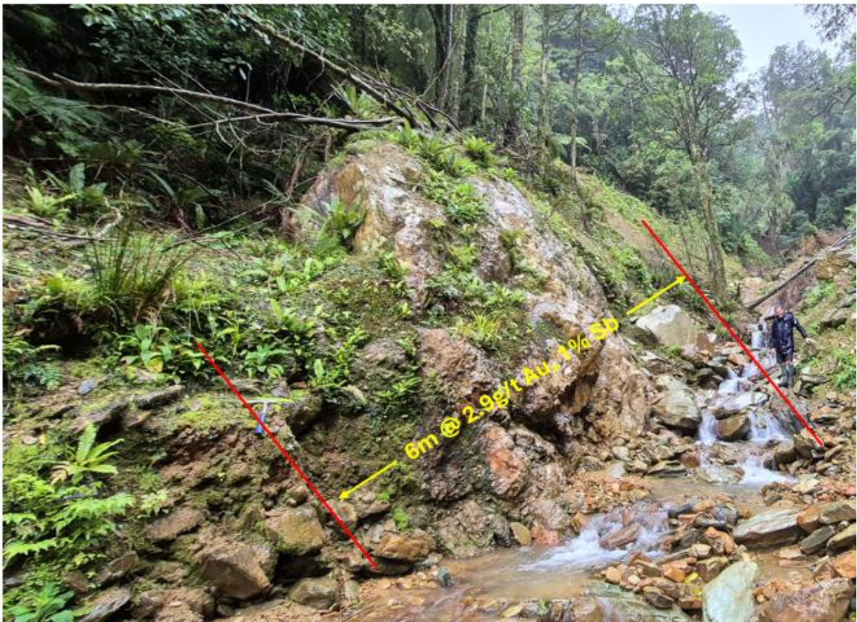
Figure 7: Maria Reef outcrop (125mRL) at the bottom of the Endeavor Inlet mine (True width of 6m @ 2.9g/t Au and 1% Sb).
