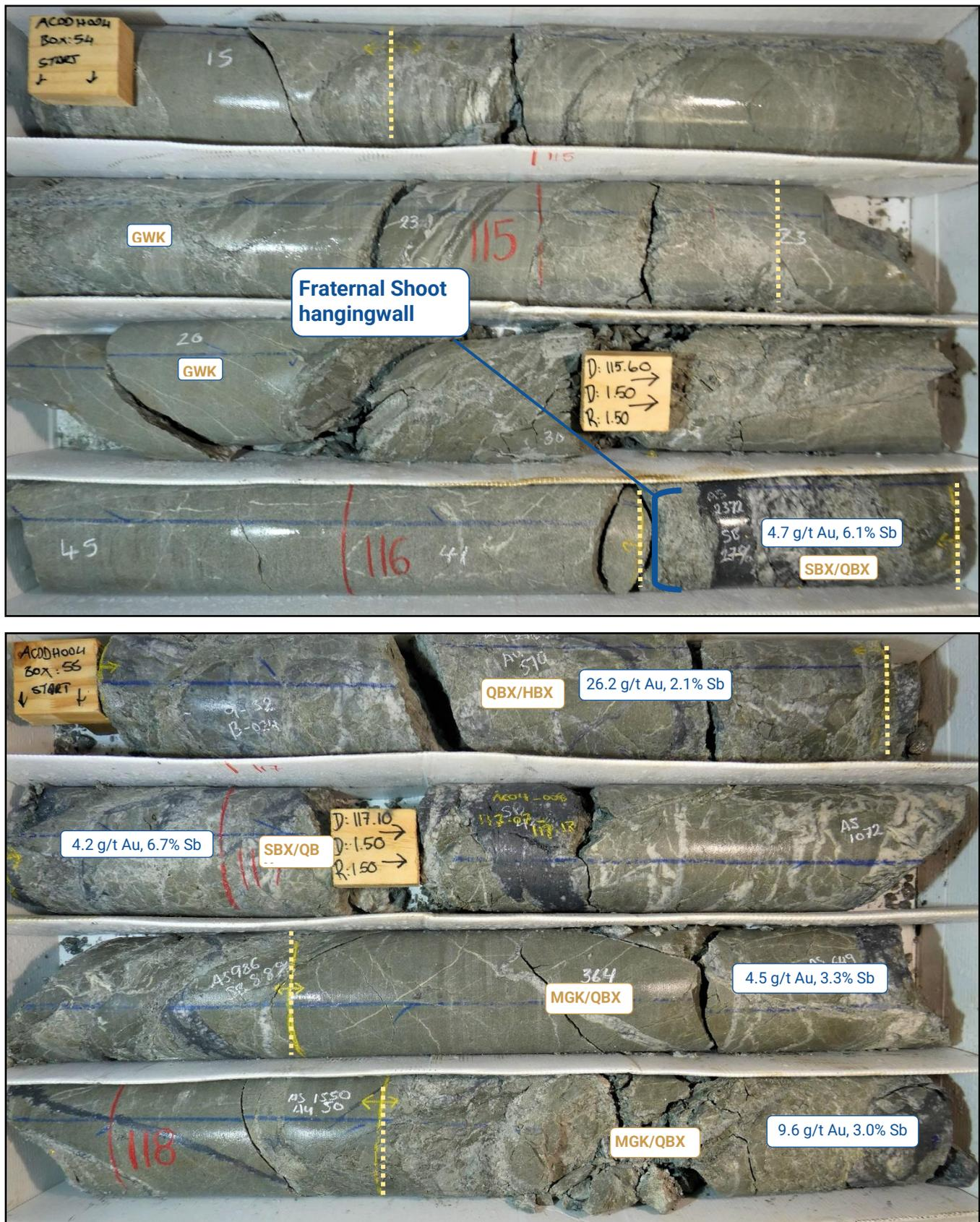
Figure 5a. Fraternal Shoot intersected in AXDDH004 116.2m – 118.4m. (SBX - stibnite cemented breccia, QBX – quartz breccia, HBX – host rock breccia, MGK – silicified disseminated arsenopyrite mineralised greywacke, MAR - silicified disseminated arsenopyrite mineralised argillite).
