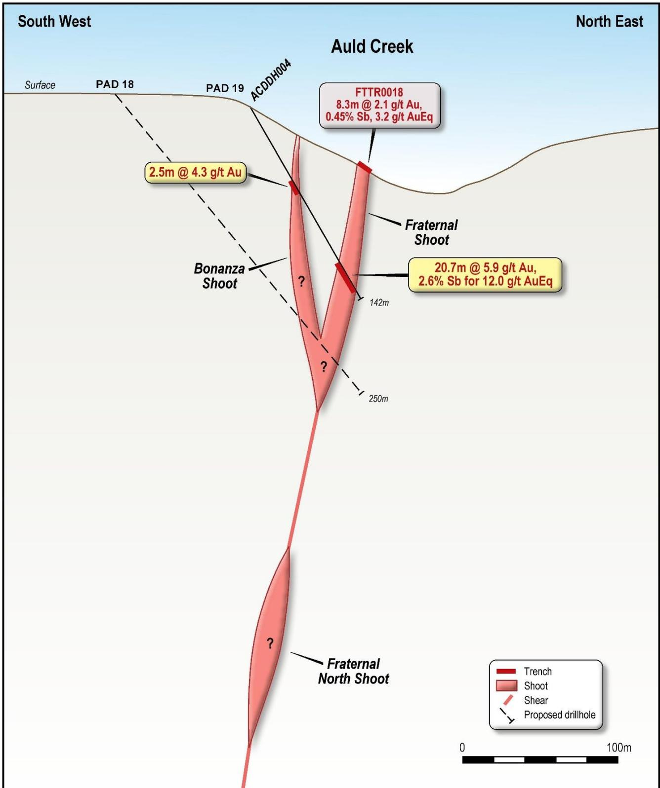
Figure 4. Auld Creek schematic cross section ACDDH004.
