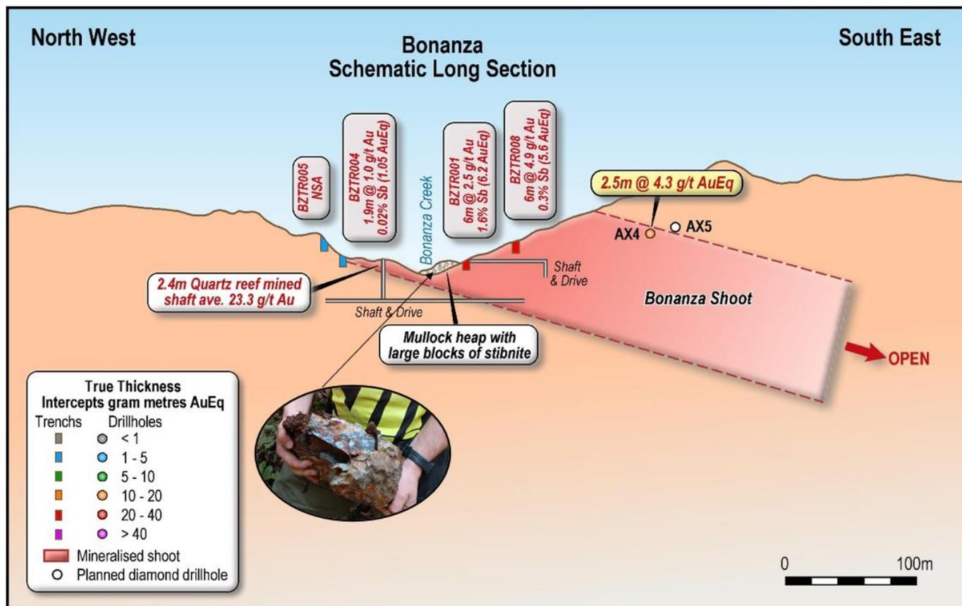
Figure 6. Bonanza N-S schematic long section.
