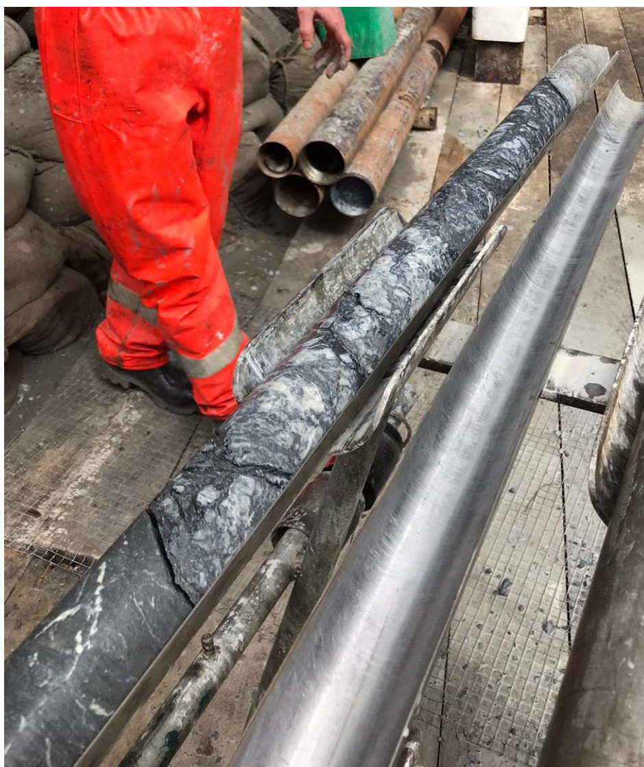
Figure 4. Quartz breccia intersected in BR44 with dike (light green) at bottom of the core.
