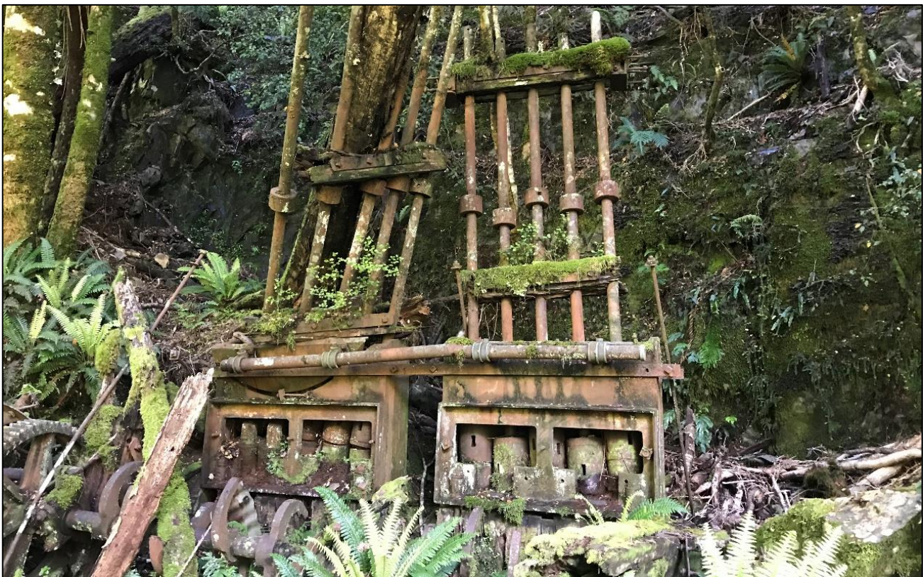
Figure 3. United Victory stamper battery found by Siren Geologists.
