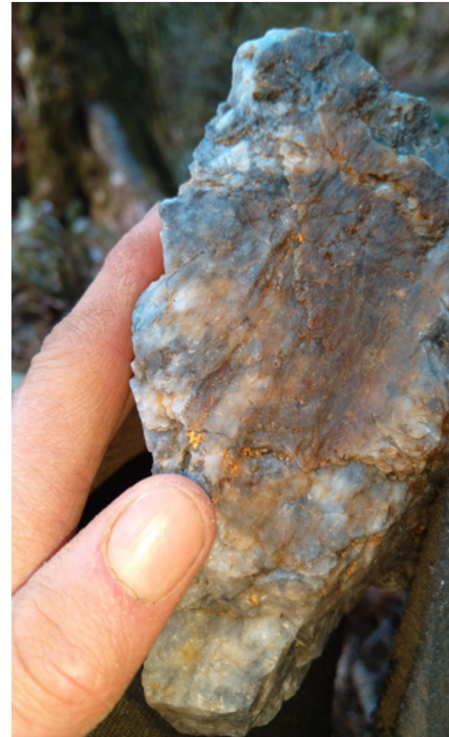
Figure 21. Quartz Reef with significant visible gold in the United Victory reef.
