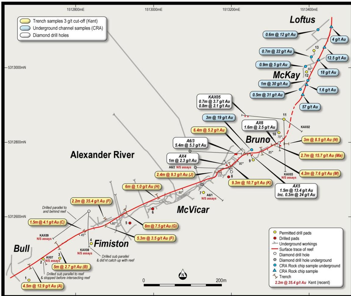
Figure 2. Alexander River prospect showing historical trenching and diamond drilling results, the current permitted drill pads (yellow dots) and used drill pads (red dots).
