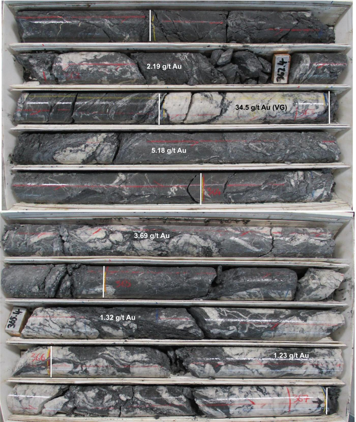
Figure 7. BRDDH34 core photos: 5.9m @ 4.1 g/t Au.
