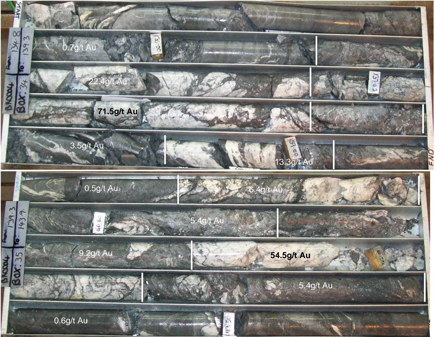
Figure 5. BRDDH004 core photos: 6.6m @ 21.4g/t Au.
