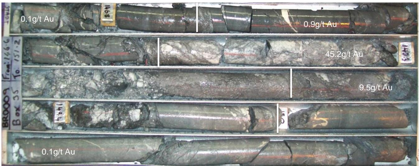
Figure 6. BRDDH009 Core photos: 3m @ 18.5g/t Au.
