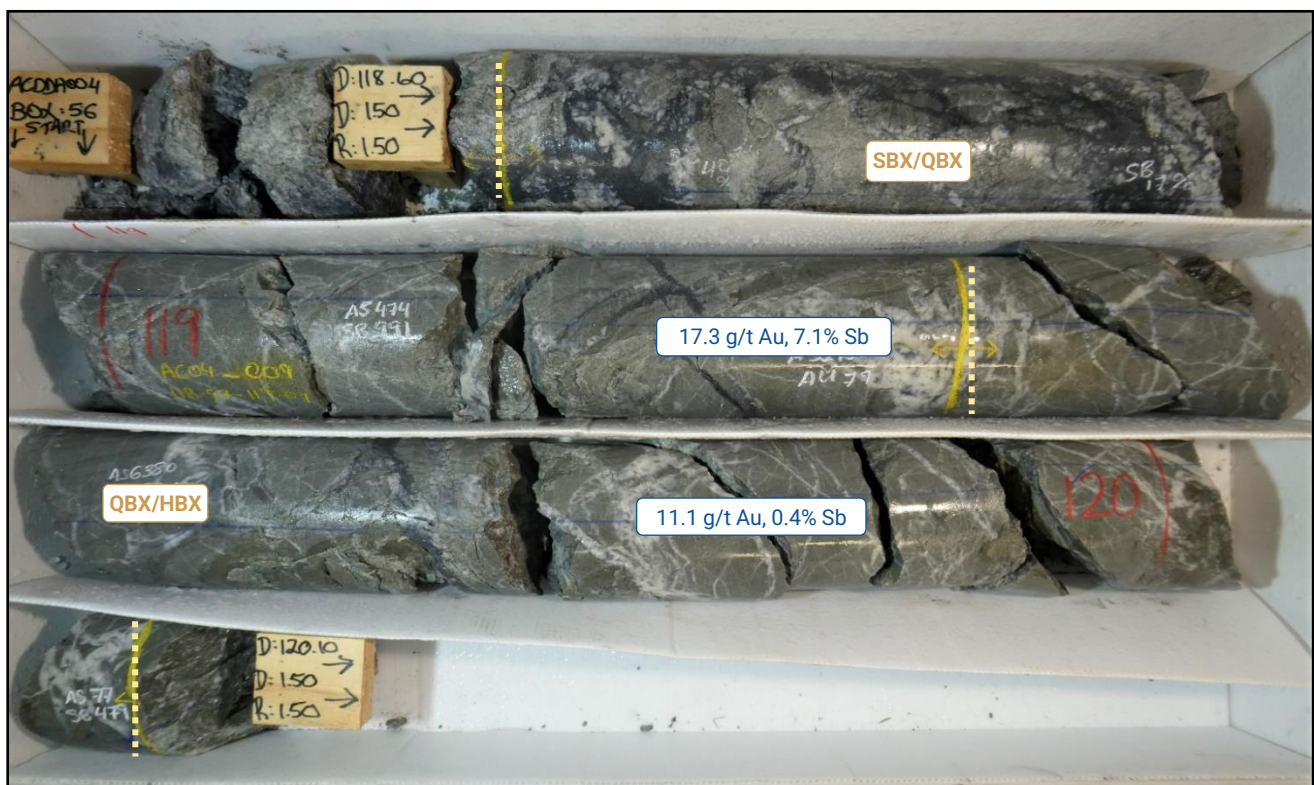
Figure 8. Fraternal Shoot intersected in AXDDH004 from 116.2m – 120.1m (SBX - stibnite cemented breccia, QBX – quartz breccia, HBX – host rock breccia, MGK – silicified disseminated arsenopyrite mineralised greywacke, MAR - silicified disseminated arsenopyrite mineralised argillite).
