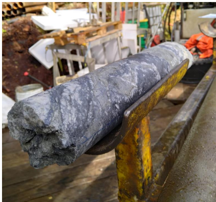
Figure 7. Stibnite (black) cemented host rock breccia from ACDDH004 at 131.4 to 131.8m that assayed 6.7g/t Au, 20.9% Sb for 56.0g/t AuEq.
