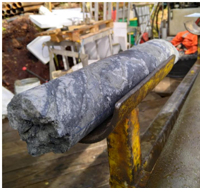
Figure 2. Stibnite (black) cemented host rock breccia from ACDDH004 at 131.4 to 131.8m that assayed 6.7g/t Au, 20.9% Sb for 56.0g/t AuEq.
